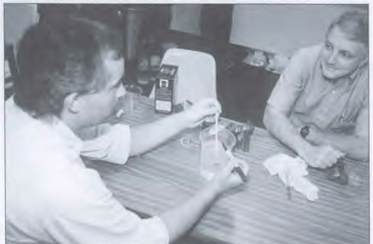
Del Spent (left), teacher at Wetakiwim, Alberta, prepares to mark the straw hydrometer which he constructed with Wayne Wasiczko, teacher at Yakima, Wash., Adventist Jr. Academy, to measure the density of different solutions.
