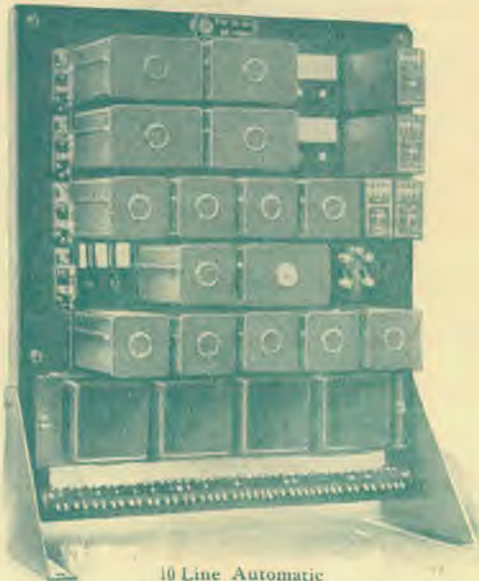
10 Line Automatic Switchboard
