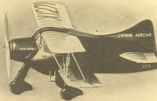
The Gwinn Aircar flying over New York. This remarkable little plane has a tricycle landing gear and foot controls similar to a car. © Keystone
