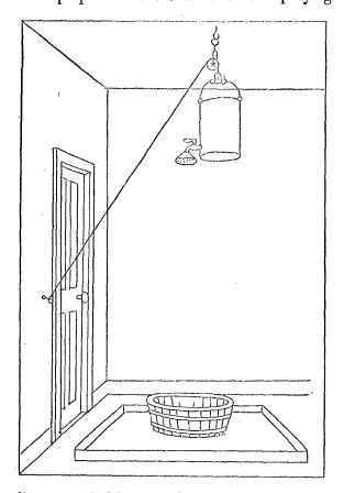
diagram will illustrate the arrangement, which consists of a shallow zinc pan three or four feet square and two inches deep, with a stiff wire in the edge of the rim. This is placed on the floor, and may contain a small tub to catch most of the falling water. In the ceiling of the room a hook is screwed, to which is attached a small pulley carrying a small rope. To one end of the rope is fastened a double wire hook to hold the bucket, and to the other end is fastened a loop
