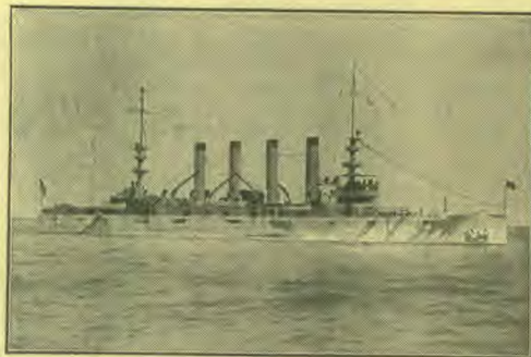
U. S. protected cruiser "Charleston." Type of five others. Displacement, 9,500 tons. Speed, 22 knots. Coal supply, 1,500 tons. Armor: belt, 4 inches; topsides, 4 in.; Deck flat, 2 in.; slopes, 3 in. Whole number of cruisers: first-class, 5; second-class, 7; third-class, 16.
