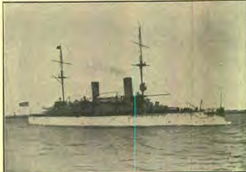
U. S. protected cruiser "Olympia." Displacement, 5,870 tons. Speed, 21½ knots. Guns: ten 5-in. rapid-fire; four 8-in.; eleven 5-in.; fourteen 6-pounders, rapid-fire; four 1-pounders, rapid-fire; two Colts. Admiral Dewey's flagship in Manila Bay, May 1, 1898.
