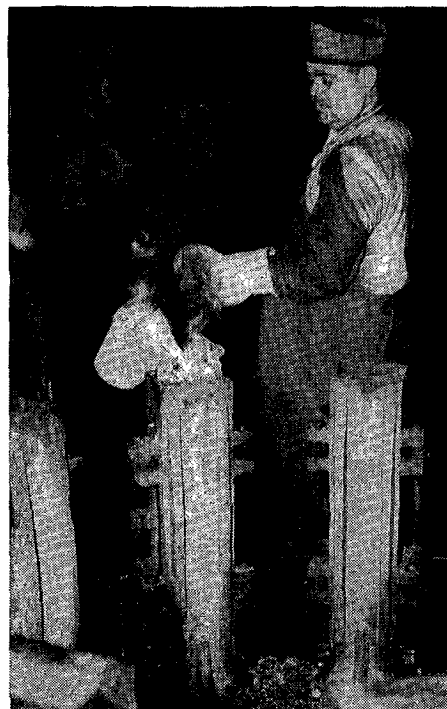
PICTURES, INC. A workman in the mint pours molten gold into a mold, to shape it into ingots for shipment to the government's new vault at Fort Knox, Kentucky.
