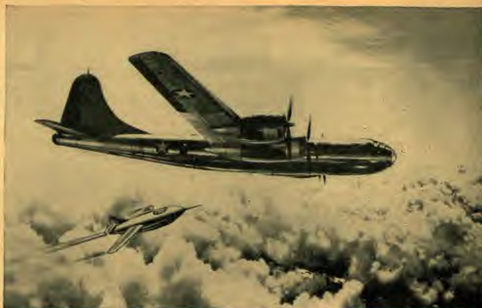
Artist's conception of the launching of the Bell XS-1, supersonic plane, from the bomb bay of a B-29. Launching aloft permits saving of rocket fuel and enables plane to travel faster than sound.
