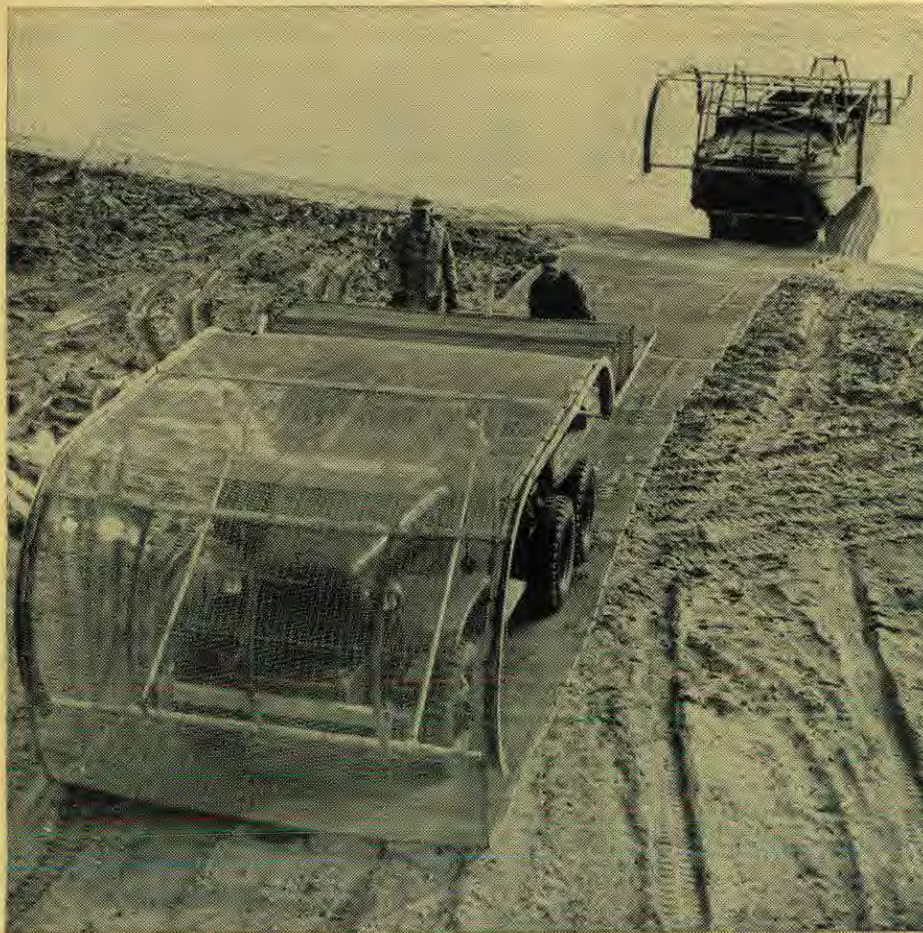
New style roadway-laying vehicles being tested by the Marine Corps for landing operations. The amphibious vehicles carry 250 feet of matting on each load.
