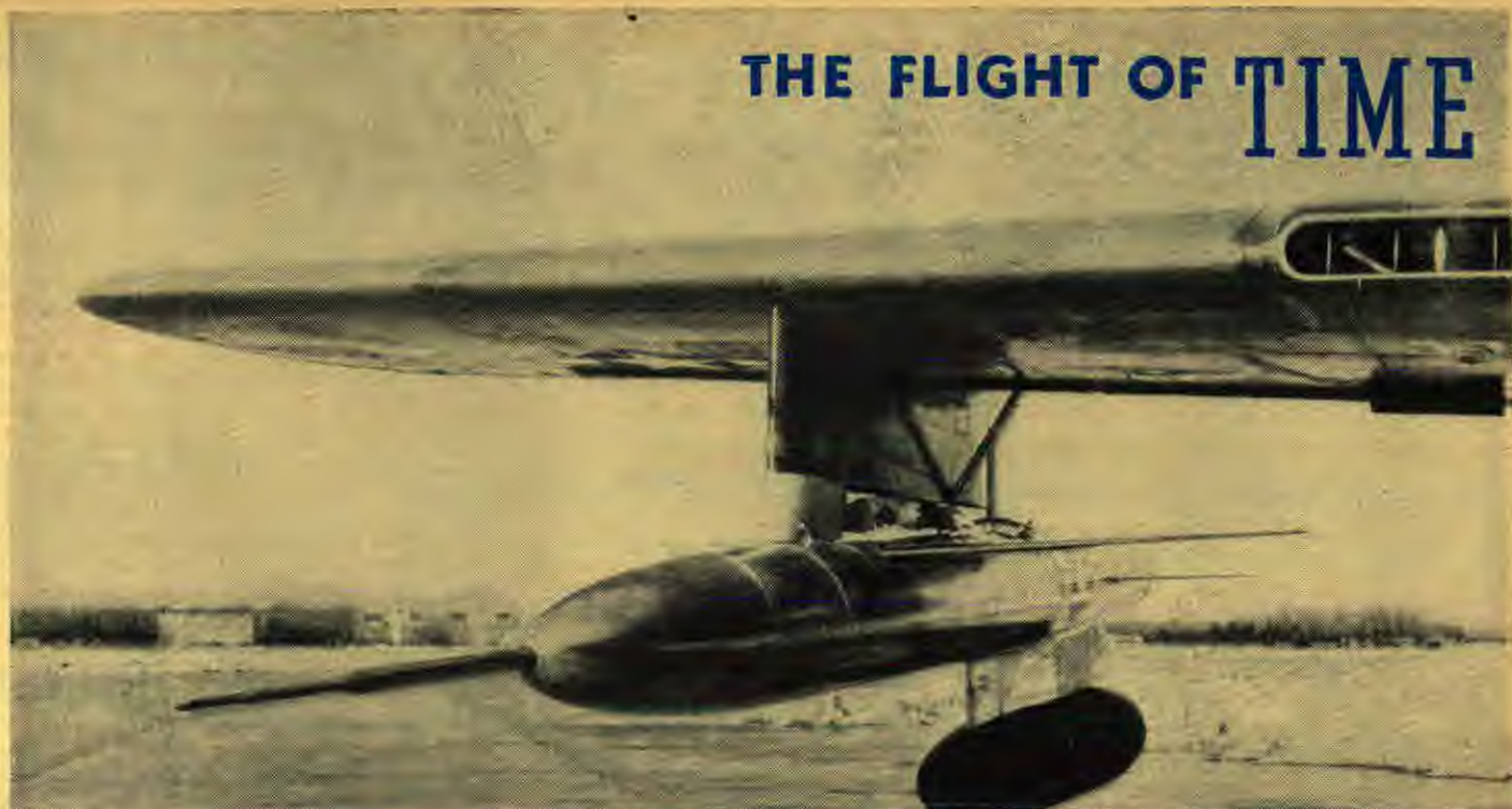
The new pilotless ram-jet missile is here seen suspended under the wing of a Black Widow fighter plane. After release it can stay aloft ten minutes while being guided to its target by radar impulses.
