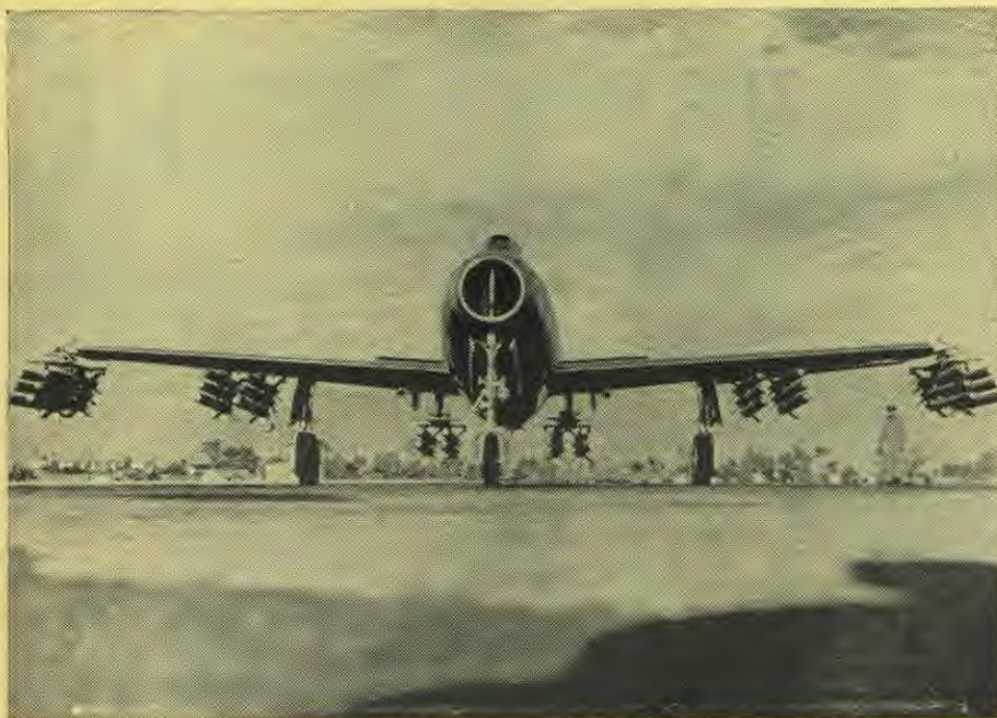
INTERNATIONAL This jet-propelled fighter-bomber, of a class known as the "Thunderjet" carries thirty-two five-inch high-velocity rockets, plus six machine guns, and flies at 600 mph.
