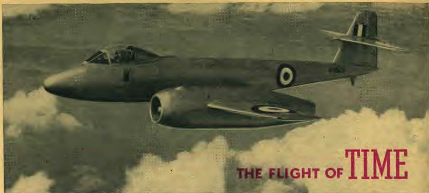
So remarkable has been the development of the jet-propelled airplane that it is claimed that each engine of the latest R.A.F. "Gloster Meteor" has about the same power as the four engines of a superfortress.
