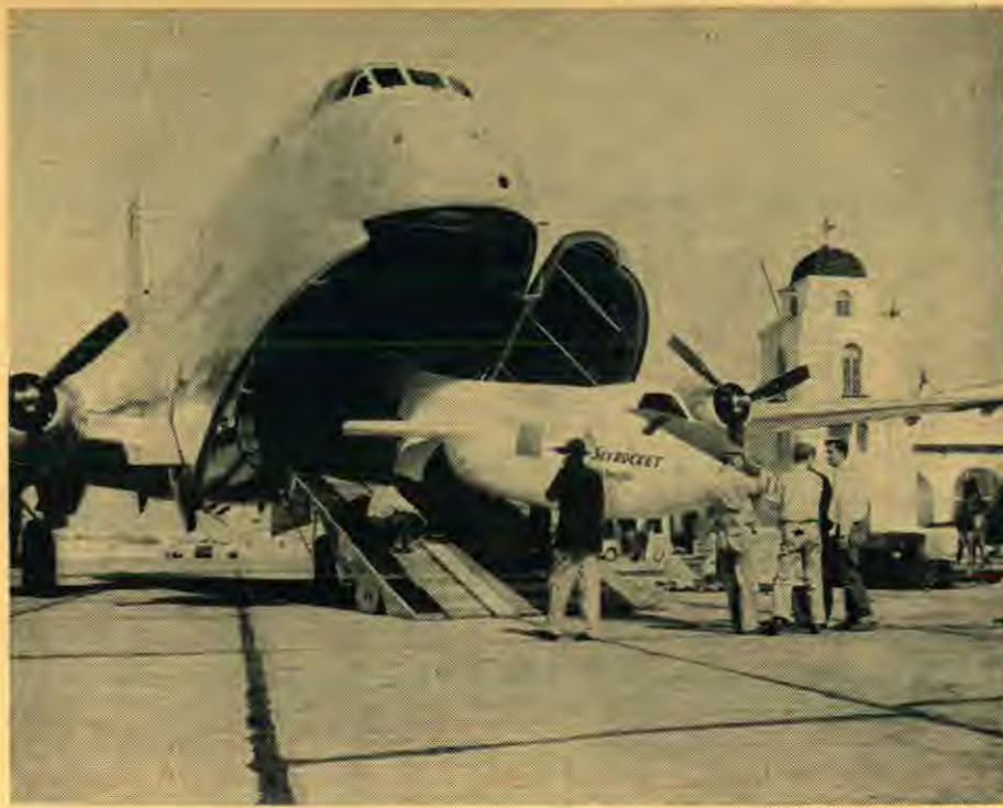
A test model of the Douglas Skyrocket is loaded on a C-124 Globemaster for a flight from El Segundo, California, to Washington, D.C.
