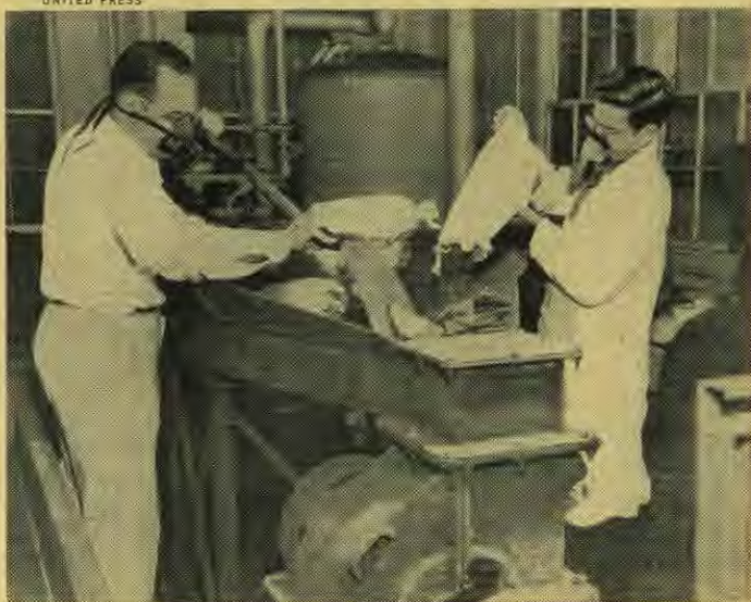
Uranium ore is put in a machine for grinding in preparation for experimental research at Oak Ridge National Laboratory.
