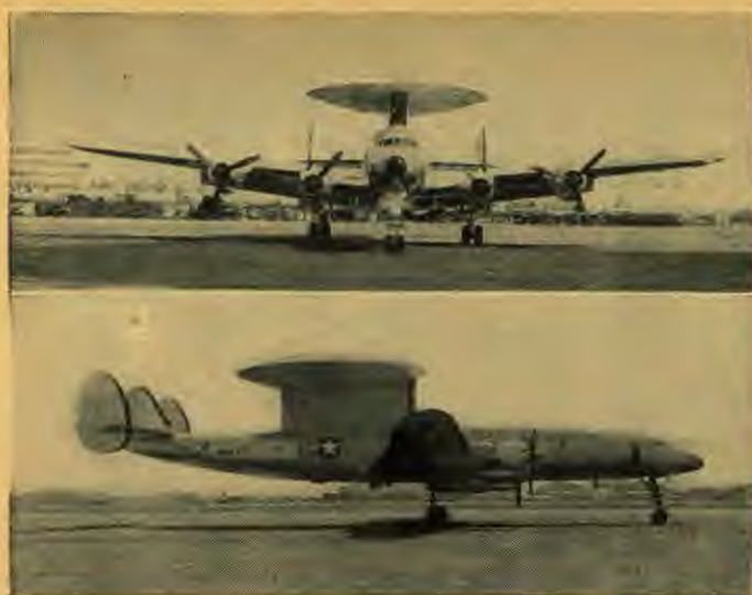
Somewhat resembling a flying saucer, a new type of radar antenna is readied for tests at the Lockheed plant in Burbank, California. The antenna is mounted on a U.S. Navy WV-2 Super Constellation like those now in operation on guard against surprise attack.
