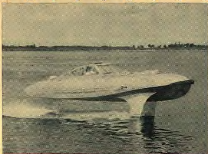
With its three legs half submerged, the wing boat developed by a German engineer races along the Elbe River at thirty miles per hour. The boat is driven by propellers on the front legs.
