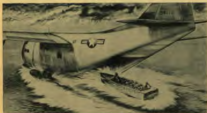
A new method of launching assault boats at beachheads from air-planes is shown in this artist's drawing. The method is made possible by hydro-lift skids that allow land-based planes to taxi on the water surface as long as forward speed is maintained. As the plane skims over the surface, a rear ramp is lowered and the wheel-equipped assault boat rolls out into the water.
