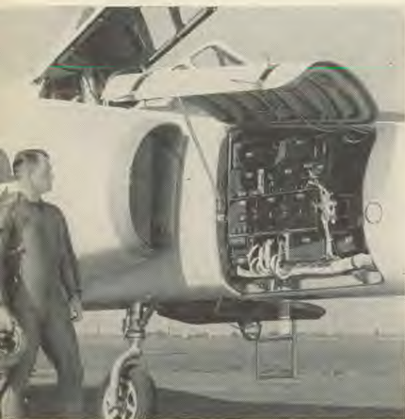
The Digitair, the first air-borne digital computer to go into actual production, is capable of making 9,600 arithmetical calculations a second. The new electronic device can automatically "fly" a plane through supersonic combat from take-off to target.
