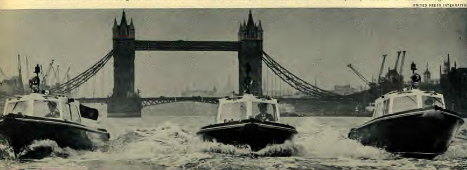
Three police speedboats zoom ahead on the river Thames, with London's picturesque Tower Bridge in the background. Three river policemen are at the controls. Made of fiber glass, the boats are economical to maintain, as this material is almost completely resistant to water damage.
