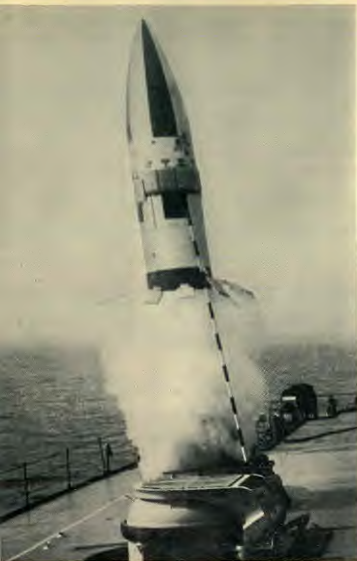
▲ An A-3 Polaris missile, one of the U.S. Navy's newest, blasts out of the missile launching tube of the U.S.S. "Observation Island" during testing.
