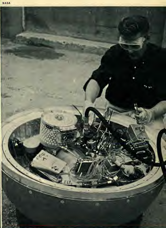
▲ A final inspection of instrumentation takes place before a capsule is sealed prior to launching. This is routine.
