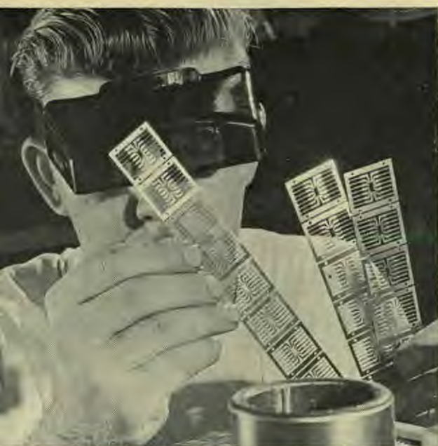
Silicon chips containing transistors, diodes, resistors, and capacitors are sealed in these lead frames which are utilized in computer and communication system industries.
