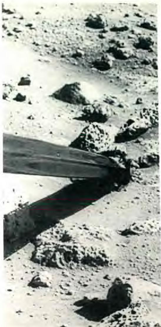
Viking's soil sampler collector arm successfully pushes a rock on the surface of Mars, October 8, 1976. The rock is shown being displaced by the arm. It is moved to the left of its original position and is left cocked slightly upward. A soil sample taken from beneath it has been sheltered from the sun's intense ultraviolet radiation.
