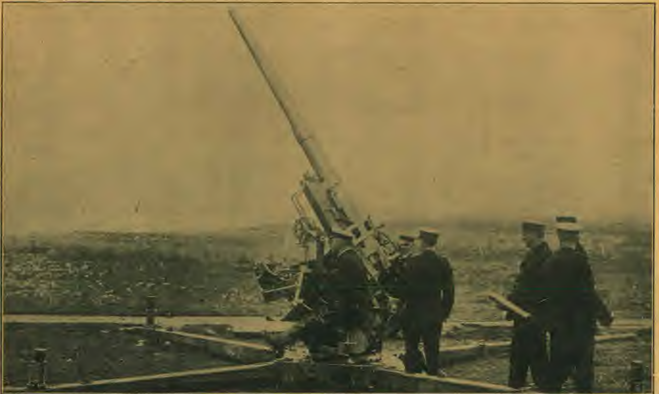
A British anti-aircraft gun capable of firing shells weighing 14 and 15 pounds at the rate of 25 rounds a minute. The gun has a vertical range of 5½ miles and a maximum horizontal range of nearly 8 miles. Even more powerful anti-aircraft ordnance has since been devised, and the nations are feverishly increasing their air forces and their anti-aircraft defences.
