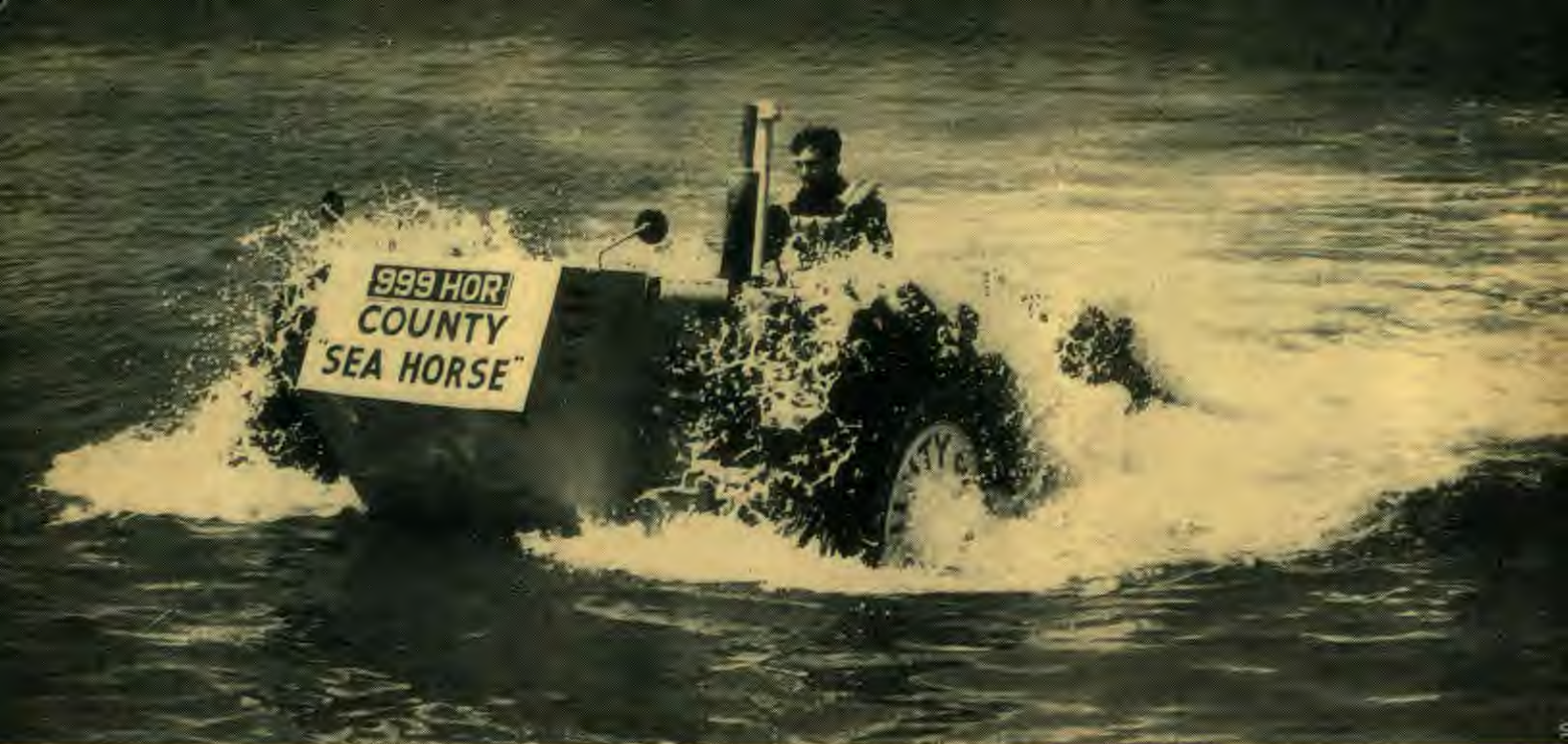
A British tractor specially designed for work on swampy ground shows its versatility by going to sea. The "Sea Horse" is equipped with five-foot-high wheels and with ballast tanks.
