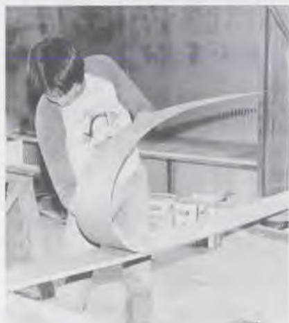
Fred Bailey laminates a board with formica at Mid-America Cabinets.
