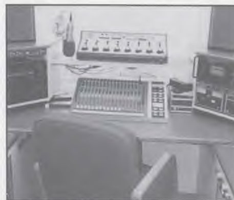
STAR production suite in Burleson, Texas. (left-Sony 8mm audio / 2 Tascam CD-501's/ Cetec & Hill mixing boards / Tandberg cassette / ITC cart / Otari 4 track reel)
