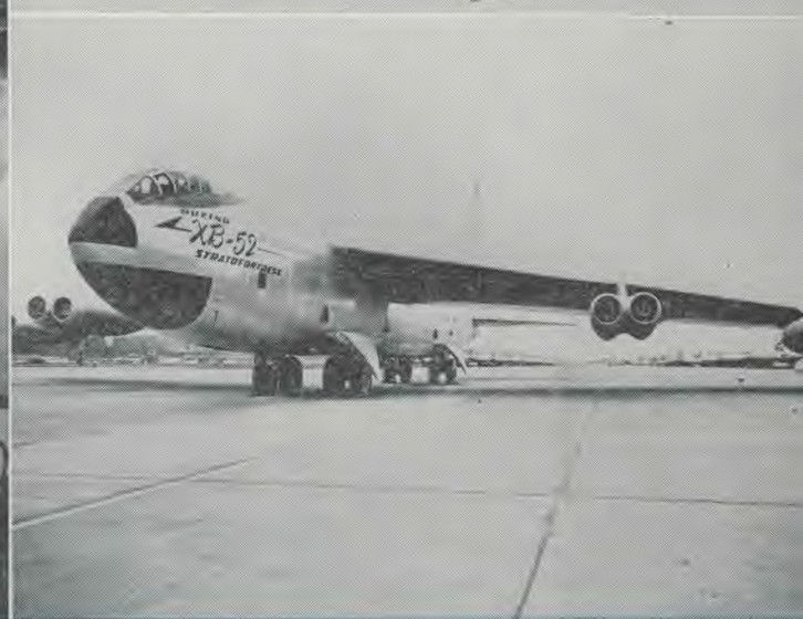
Top: America's newest jet superbomber, the Boeing B-52 Stratofortress, shown in flight. It has a wingspan of 185 feet, a length of 153 feet, and a tail height of 48 feet. Below, the giant bomber is pictured about to take off on one of several test flights. Its eight Pratt and Whitney J-57 engines are mounted in pairs in sharply raked forward pods. It has a double tandem and "protection" landing gear, as well as other unusual ultra-modern devices.
