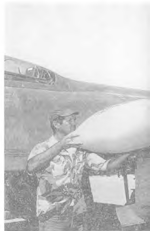
A mechanic places the fiberglass cover on the new F-94C "Starfire" fighter. The pods carry twelve 2. twenty-four already carried in the plane's nose.
