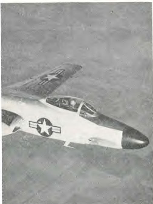
McDonnell F2H-3 Banshee now in production for an anodized finish. The silver Banshees will be in all kinds of weather during carrier operations.
