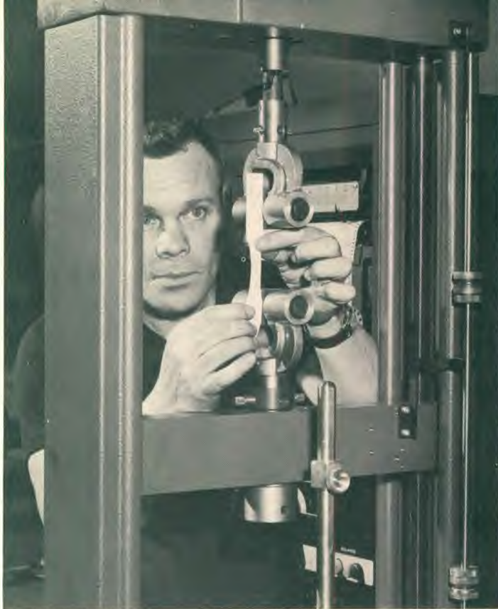
A technician of the Forest Products Laboratory is inserting paper in the jaws of a testing machine in order to determine tensile strength.
