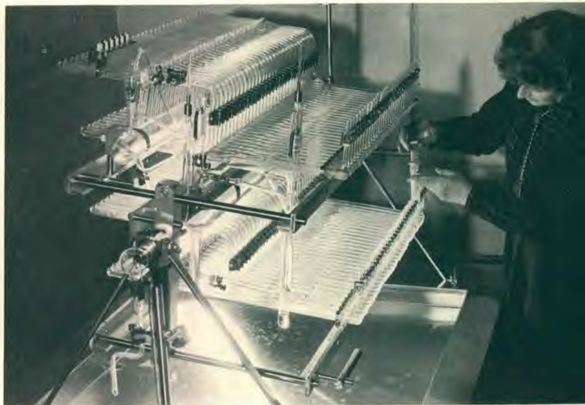
Craig extractor is used to separate flavanoids from mixture in solution.
