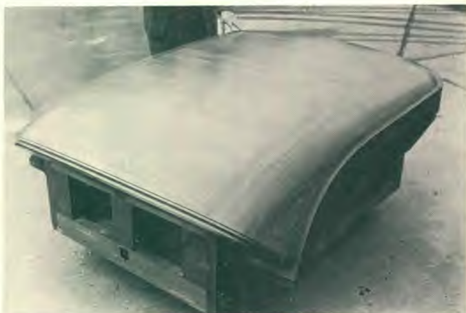
Impreg is a form of resin-treated laminated wood, and is used in making die models by the auto industry to avoid costly recarving.
