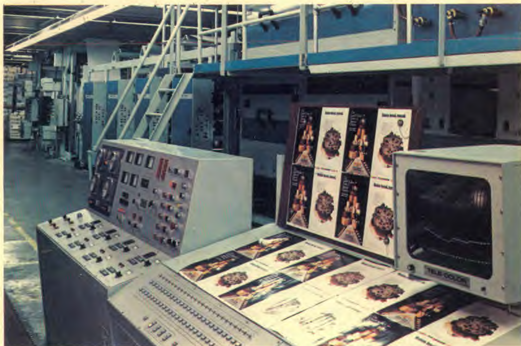
The Washington hand press, left, was used to publish the Review from 1852 until 1857. It took three days to print each issue on that press. In February, 1976, a new web press like the one on the right will print the Review in six hours, at 32,000 printing impressions an hour.
