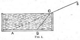
Careful experiments have proved that the velocity of light is less in a dense than in a rare medium. Light travels more rapidly in air than in water, since air is less dense than water. Remembering that the velocity of light in air and in water is diferent, we may get a fairly clear idea of why light is refracted without entering into the mathematical discussion of the matter, though it is only by mathematics that we can prove what I shall here state.
