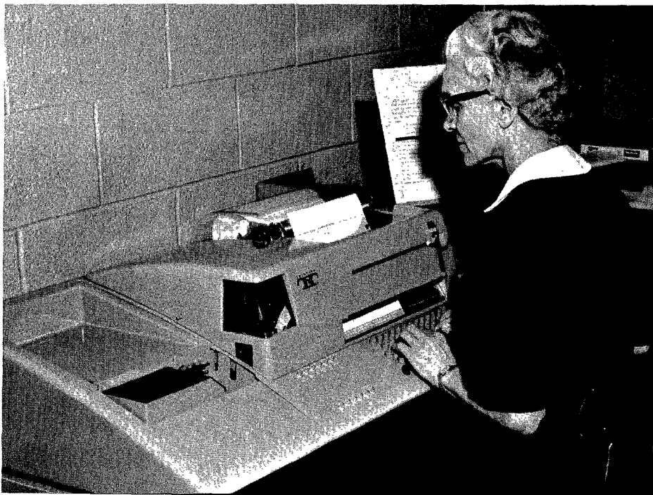
Mrs. Promise Sherman, REVIEW editorial secretary, operating the TWX machine, sending reports of the conference proceedings from the editorial offices in Detroit. The taped transmission reaches Washington at 100 words a minute.
