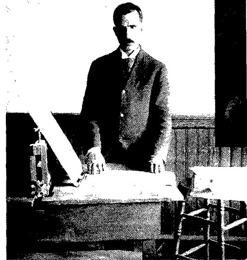
A LIFE-CHANGING CREATION: Austin Wilson demonstrates his braille press, fashioned from a hand-operated clothes wringer. Wilson converted the wringer into a press and mounted the device on a table, circa 1900.
