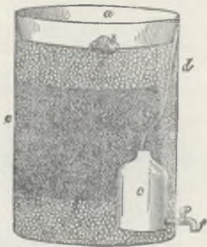
FIG. 3. Simple Form of Filter, for household use. a. Water-pan, or reservoir; b. Sponge; c. Jug to receive filtered water; d. Gravel; e. Charcoal; f. Faucet.
