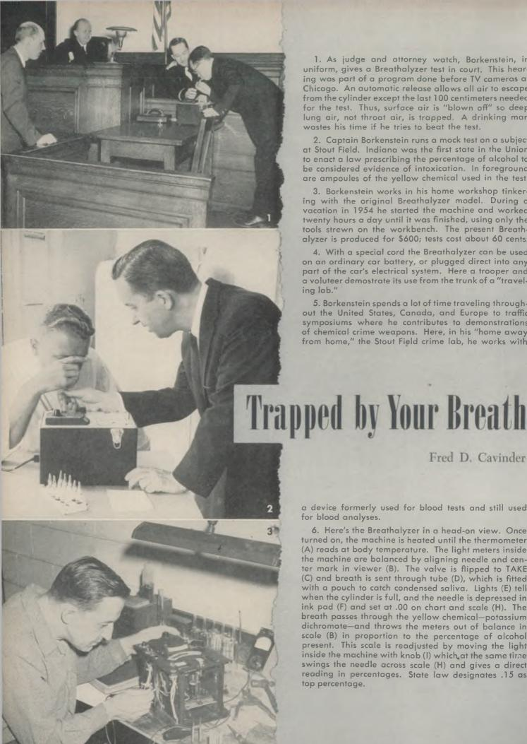
1. As judge and attorney watch, Borkenstein, in uniform, gives a Breathalyzer test in court. This hearing was part of a program done before TV cameras at Chicago. An automatic release allows all air to escape from the cylinder except the last 100 centimeters needed for the test. Thus, surface air is "blown off" so deep lung air, not throat air, is trapped. A drinking man wastes his time if he tries to beat the test.
