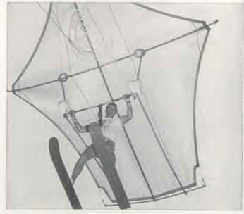
Ken Tibado, of Lake Wales, Florida, demonstrates the simplicity of a kite's design. He holds the extreme ends of the bar in order to maintain the best balance and control. All fittings holding the framework and cables in place should be double-checked when assembling.
