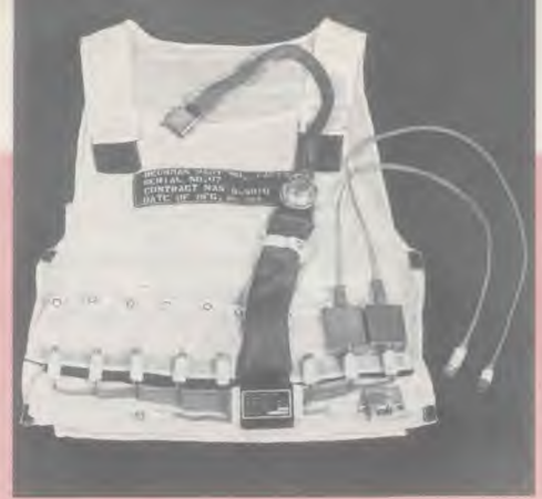
This garment worn by the Gemini astronauts has attached to it simple medical instruments capable of relaying to the aerospace doctor on the ground complicated medical data on the astronauts in orbit.
