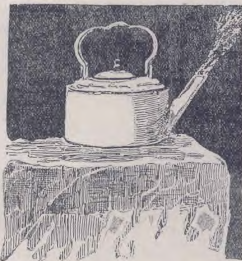
A kettle containing liquid air at 312° below zero, boiling on a block of ice. The temperature of ice is 32° above zero. There is therefore a difference in temperature of 344°.
