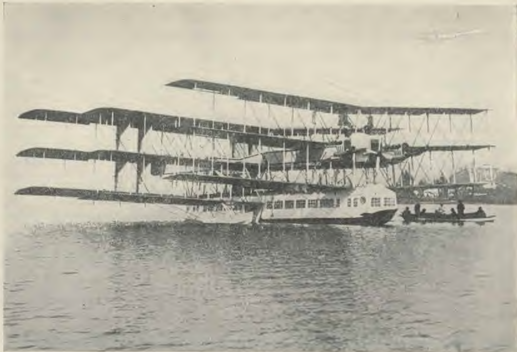
The largest airplane ever built. This giant flying boat was provided with cabin accommodations for one hundred passengers. The Italian inventor proposed to cross the Atlantic to America in her, but she was wrecked during a trial trip on Lake Maggiore, Italy.
