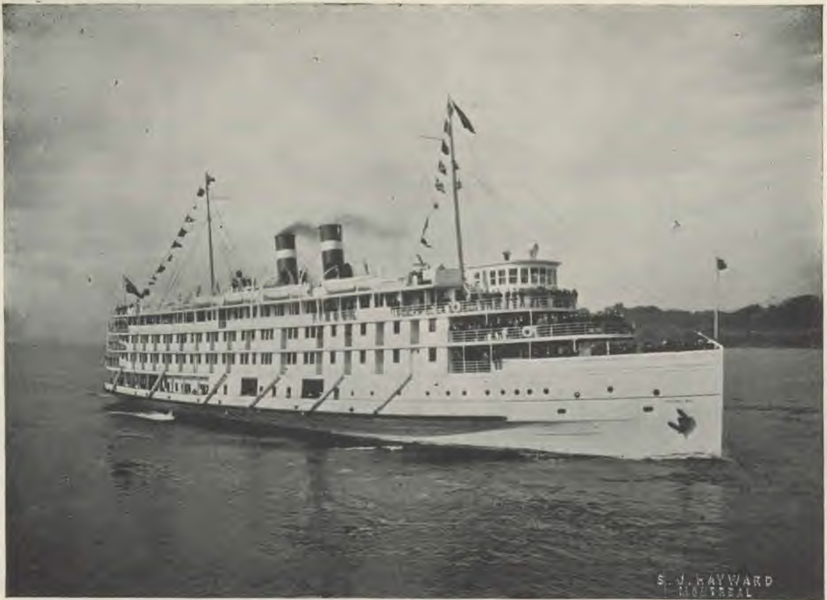
The new "Richelieu" leaving Montreal on her trial trip June 9. She is the largest passenger carrier of the Canada Steamship Lines, Ltd.; is 332 feet long, burns oil for fuel, and attains a speed of twenty miles an hour.
