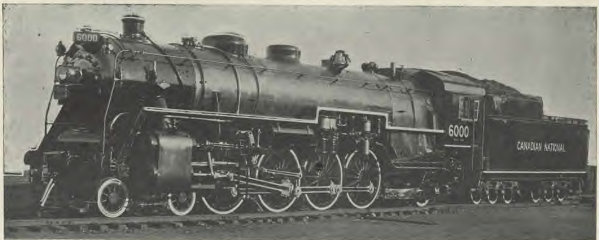
The largest passenger engine in Canada. The overlength of this engine and tender combined is 90 feet; total weight, 290 tons. Sixteen of these engines are being built.
