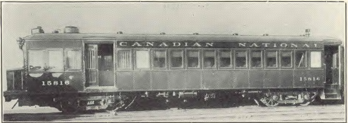
Capreol-Parry Sound motor car. This is a new form of equipment that helps the railroads to meet bus-line competition.
