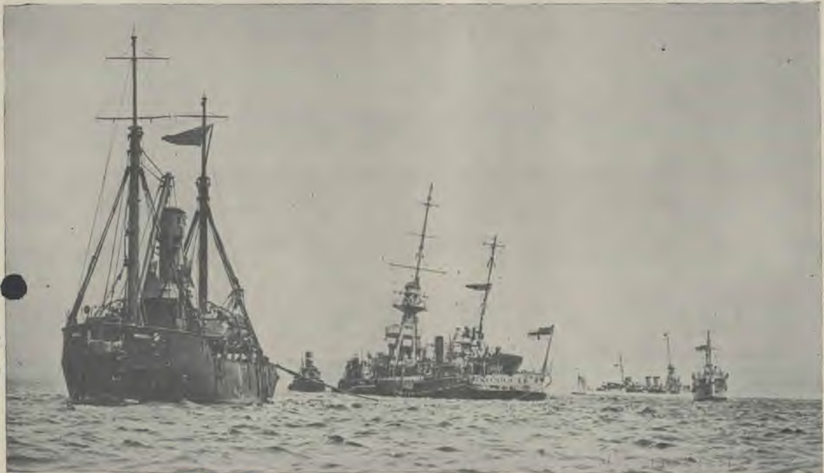
The refloating of H. M. S. "Dauntless." Although it was thought impossible to salvage the ship, she was refloated just nine days after she struck the rocks. The illustration shows the salvage ship "Reindeer" hauling her off the rocks with a fifteen-inch hawser.
