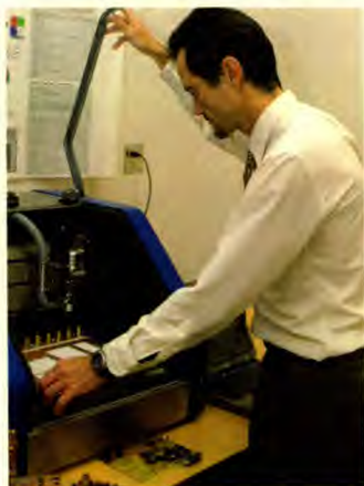
School of Computing Dean Richard Halterman demonstrates how a milling machine is used to fabricate custom circuit boards.
