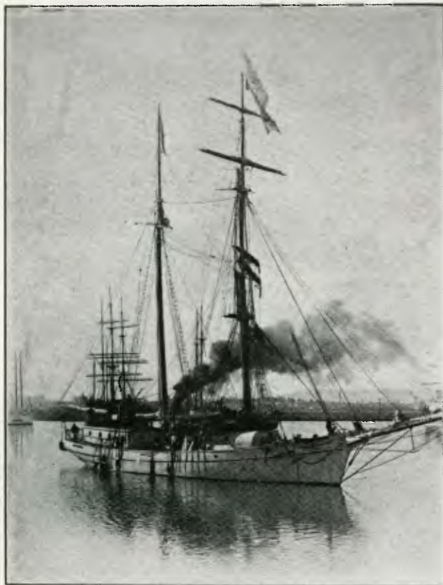
By 1892 the cabin, forecastle, and galley were brought above deck and auxiliary power was added to help the ship in and out of ports.
