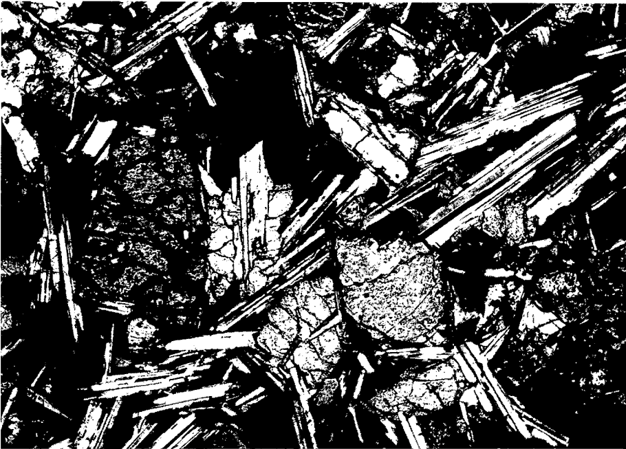
B. Microphotograph of a coarsely crystalline basalt from Umm al-Jamal . Mineralogy: olivine (large angular crystals), plagioclase (elongate lathes), pyroxene (inter-crystalline area). (40 ×)
